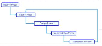
**Five-Phase Waterfall Model.** It extends the four-phase model with the reuse of existing ontological resources as they are.
