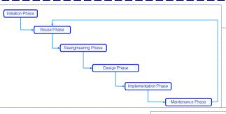
Six-Phase Waterfall Model. It extends the five-phase model with the Reengineering Phase. It allows the re-engineering of ontological resources and non-ontological resources (NORs). It may occur that several knowledge resources are transformed into ontologies in the reengineering phase.
